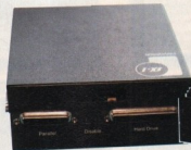
You may also fit an external IDE drive, but it must have its own power supply. While the serial port is not the standard Amiga DB25 connector, the 9-pin IBM AT style connector is more than adequate
